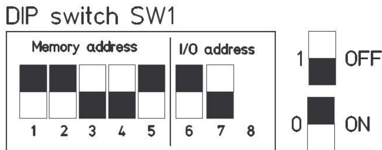
Figure 1 DIP switch SW1
